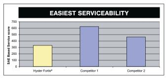
Society of Automotive Engineers (SAE)-based rating evaluating speed and difficulty of over 30 service routines. Lower score indicates easier serviceability.
