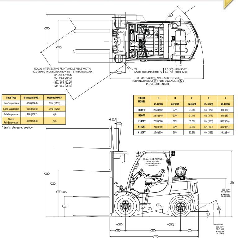
Circled dimensions correspond to the line numbers on the tabulated chart inside the Technical Guide. Dimensions are in inches (millimeters).
