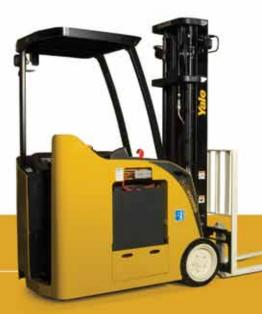
hip, arm and knee support and offers the operator a cooler workspace. The high backrest support provides the operator both comfort and protection. The noticeably large floor has room for movement. The shock dampened suspended operator's compartment floor with full 3/4" thick cushioned floor mat absorbs vibration and minimizes fatigue. The brake pedal design allows for an easy entrance and exit into the operator compartment.
