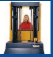
A large safety glass windshield provides maximum unobstructed visibility and prevents contact with moving mast components. The Yale Hi-Vis mast provides excellent visibility and smooth mast staging for stepless lifting and lowering of the mast. Yale features a non-retractable operator tether with a full body harness as standard.
