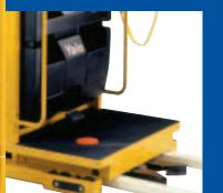
The operator has a low-fatigue, highly productive work station that features low step height, wide cushioned floor, a foot switch position that promotes a natural and comfortable stance, plus a one-inch thick padded rubber floor mat for supportive comfort. The Yale order selectors and straddle selectors have a pallet lock mechanism to secure the pallet in place.
