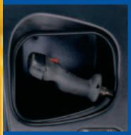
The multi-function control handle provides improved ergonomics for operator comfort. It has a thumb-actuated control for the single speed lift/lower functions on the OS-EC and variable speed lift/lower functions on the OS/SS-BE with a trigger-style horn button on both. The handle can be rotated to one of three positions for a comfortable operating stance.
