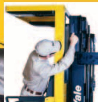
*Side thrust adjustable mast allows the technician to quickly and easily adjust all mast channel rollers in the field to compensate for wear. Adjustment can be accomplished without special tools or mast disassembly. Trunnion mounted mast allows for easy mast removal. The OS-BE is shown with the optional light package.*
