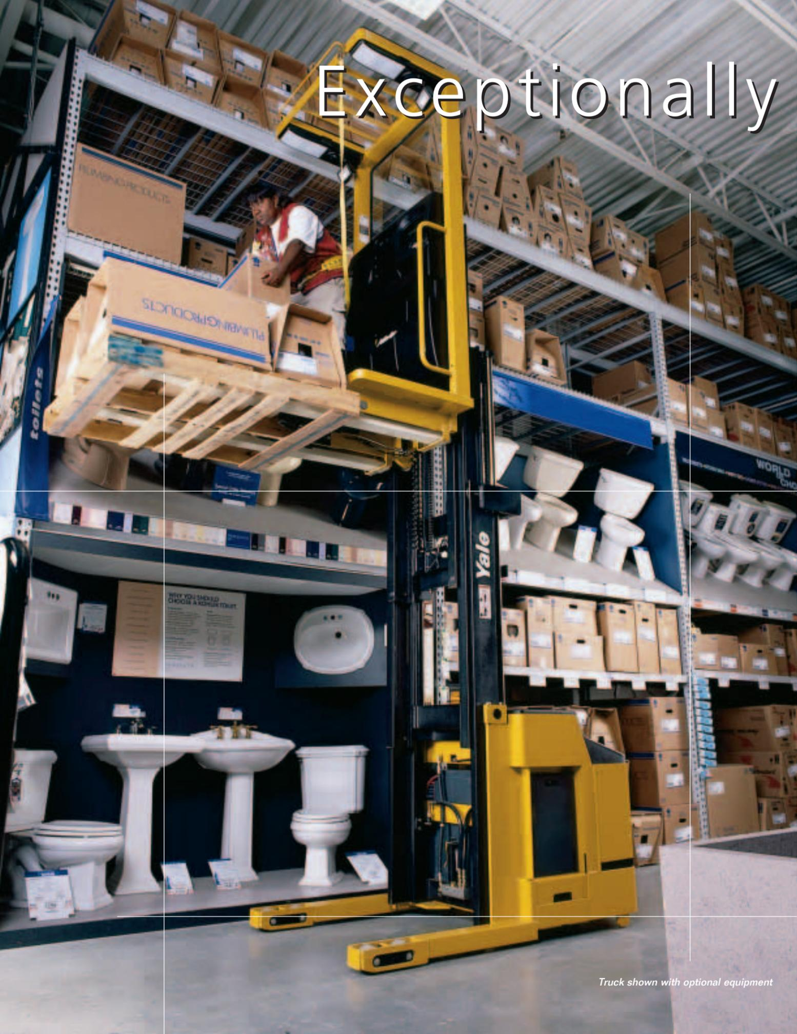
A yellow Yale order selector truck is shown in a warehouse setting. The truck is positioned in front of high industrial shelving units filled with cardboard boxes. A worker is visible on the platform of the truck, reaching for a box. The truck has a wooden pallet on its forks. The background shows more shelving units and a display area with white ceramic fixtures like sinks and toilets. The text 'Exceptionally hard working' is overlaid on the top left of the image.
