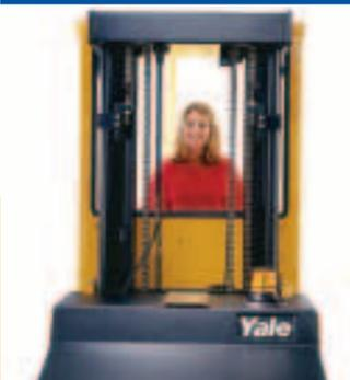
A large safety glass windshield provides maximum unobstructed visibility and prevents contact with moving mast components. The Yale Hi-Vis mast provides excellent visibility and smooth staging for stepless lifting and lowering of the mast. Yale features a non-retractable operator tether with a full body harness as standard.
