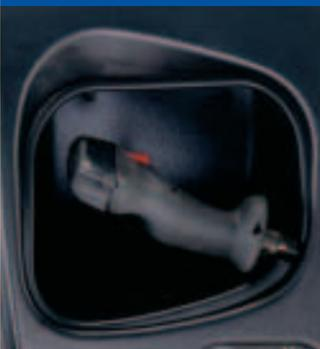
The multi-function control handle provides improved ergonomics for operator comfort. It has a thumb-actuated control for the single speed lift/lower functions on the OS-EC and variable speed lift/lower functions on the OS/SS-BE with a trigger-style horn button on both. The handle can be rotated to one of three positions for a comfortable operating stance.
