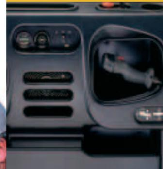
*The backlit alphanumeric display is compatible with the Controlled Area Network (CAN) communications system. It allows the display of fault messages and also serves as a battery discharge indicator and hour meter. This also allows technicians to use the display as a troubleshooting device. The handle is also used in conjunction with the alphanumeric display to set truck performance parameters. Shown with upper-body ventilation fan.*
