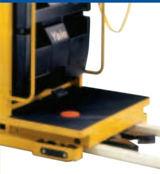
The operator has a low-fatigue, highly productive work station that features low step height, wide cushioned floor, a foot switch position that promotes a natural and comfortable stance, plus a one-inch thick padded rubber floor mat for supportive comfort. The Yale order selectors and straddle selectors have a pallet lock mechanism to secure the pallet in place.
