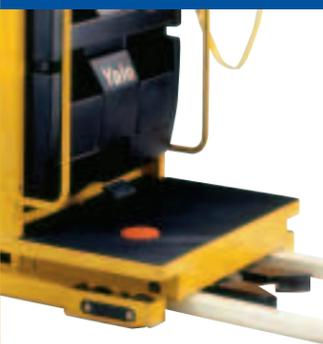
The operator has a low-fatigue, highly productive work station that features low step height, wide cushioned floor, a foot switch position that promotes a natural and comfortable stance, plus a one-inch thick padded rubber floor mat for supportive comfort. The Yale order selectors and straddle selectors have a pallet lock mechanism to secure the pallet in place.
