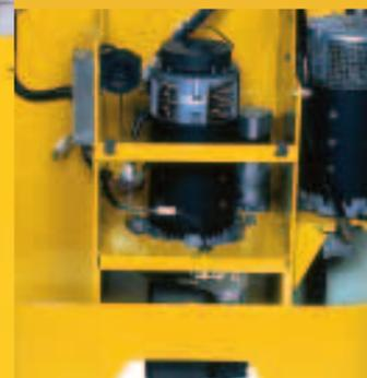
*The stationary drive motor eliminates power cable flexing improving cable reliability. The direct drive steering system uses a maintenance-free brushless DC motor. The Auto Deceleration System uses the drive motor to slow down the truck which reduces brake wear and minimizes flat spots on the drive tire. The OS-BE is shown.*
